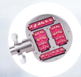
Fig. 3 The CAM-processing of the denture teeth is done similarly to the basal and circular construction.
