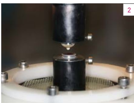
Fig. 2 The pin-on-block (POB) wear test was conducted on eight different samples per product with a steatite ball.
