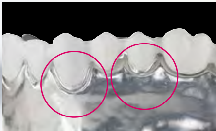
Fig. 1a Visual fit check after sintering process of the VITA YZ T using a control model.
