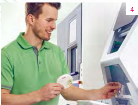
Fig. 4 The magazine of a CAM unit is equipped with a VITA YZ ST blank.
