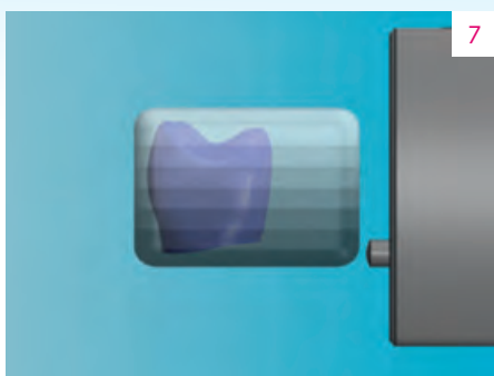
Fig. 7 The shade gradient could be controlled in a targeted manner by vertically positioning the crown in the virtual blank.
