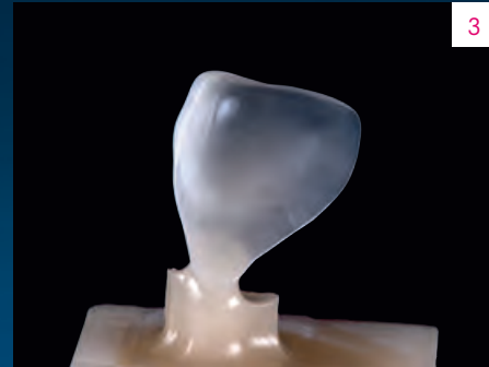
Fig. 3 The high-precision result after the grinding process with CEREC MC XL.
