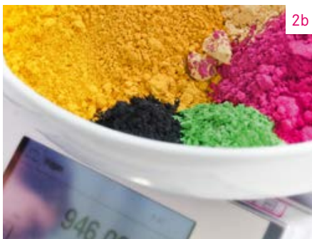
Fig 2a-b Sample representation of the visual inspection of the shade fidelity of a VITA LUMEX AC sample crown to the VITA shade standard, and for the implementation of a shade formula using ceramic powders mixed with color pigments.
