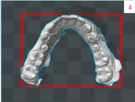
Fig. 4 The virtual model of the lower jaw was used as the basis for the production of a control model using additive manufacturing.
