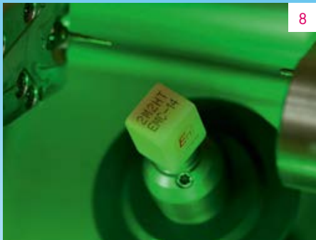
Fig. 8 The highly translucent, hybrid ceramic block in the color 2M2 clamped in the grinding machine.
