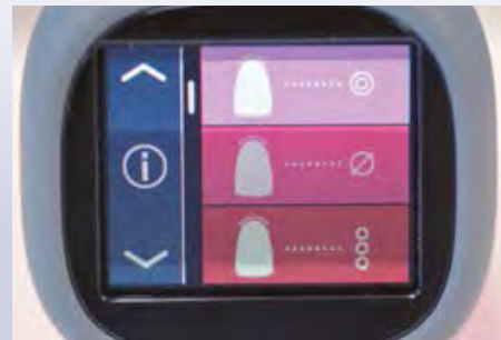
Fig. 1 Main menu of the OLED color touch display. Shown here: Basic shade measurement, average measurement and tooth area measurement.
