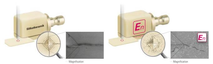
Fig. 1&2 Source: Internal study, VITA R&D, Vickers indentation, left silicate ceramic, right hybrid ceramic (1)
