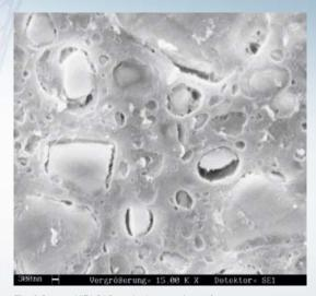
Fig. 2 Source: VITA R&D, etched composite surface Composite: polymer with ceramic filler particles
